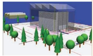
At the click of a button, Plant Simulation's bottleneck analyzer shows the utilization of resources, thus indicating bottlenecks as well as underworked machines.
